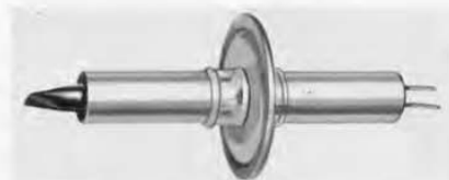
Figure 3. The 5675-type pencil tube used in the Type 1218-A Unit Oscillator.
