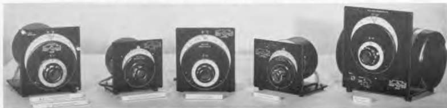
Figure 2. Group of Unit Oscillators covering a frequency range of 0.5 to 2000 megacycles. The lengths of the bars in front of the units indicate their frequency coverage on a logarithmic scale.
