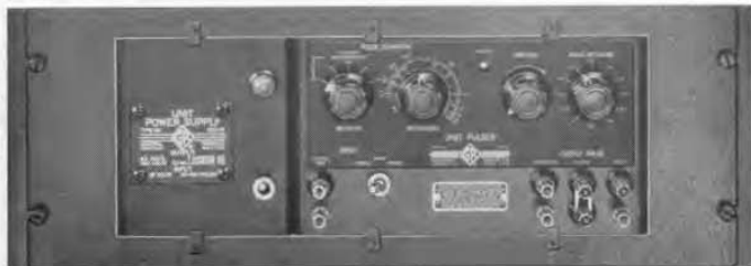
Figure 1. View of the Type 1217-A Unit Pulser and the Type 1203-A Unit Power Supply mounted in a Type 480-P4U3 Relay-Rack Panel.
