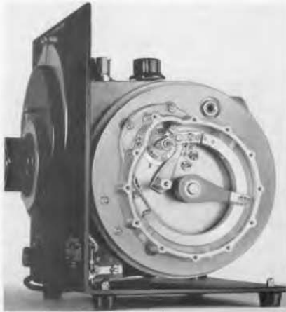
Figure 4. View of the right-hand end of the oscillator assembly with cover removed to show the cathode line.
